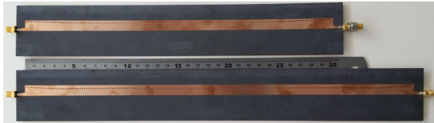
Figure 3.13. Photograph of the fabricated antennas. Photographs are shown for the antennas optimised for low sidelobe level (top) and wide null (bottom).
