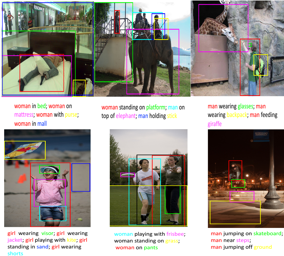
Figure 7.4: Qualitative examples of the predicate detection. The color of human and objects in the phrases correspond to the color of the bounding boxes. We only predict the interactions between the ground-truth bounding box pairs.
