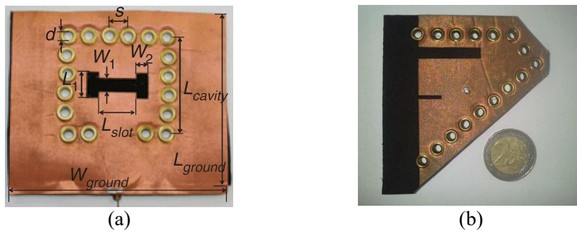
Figure 2.23. Textile antennas using metallic eyelet vias. (a) A textile cavity-backed slot antenna (adapted from [20]) and (b) a textile HMSIW-based antenna using metallic vias to form a shorting wall (adapted from [22]).
