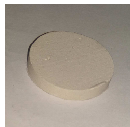
Figure 9.10. A flexible DR prototype. A DR prototype realized in PDMS and ceramic powder using the mold shown in Fig. 9.8.
