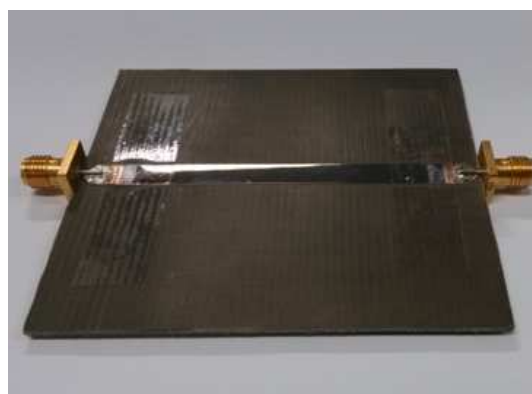
Figure 3.29. The microstrip line test jig. The test jig used to measure transmission coefficients of the microstrip lines with 1-layer and laminated PEDOT conductor.
