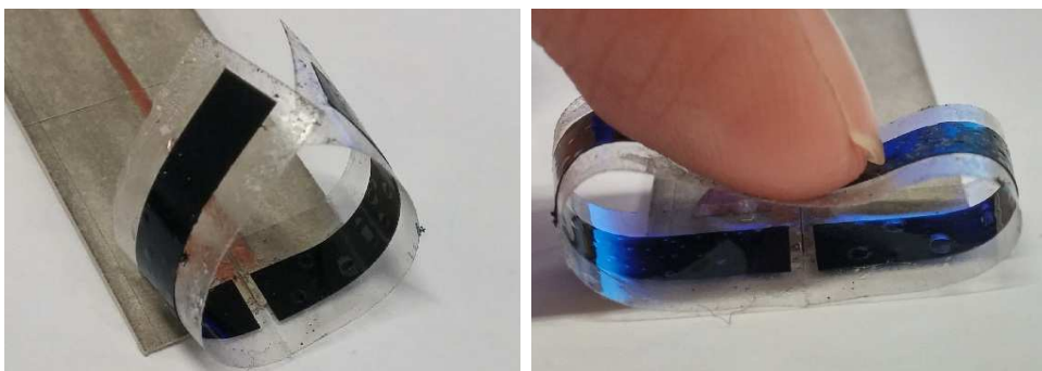
Figure 3.23. Bent dipole antenna. PEDOT antenna in two bending configurations.
