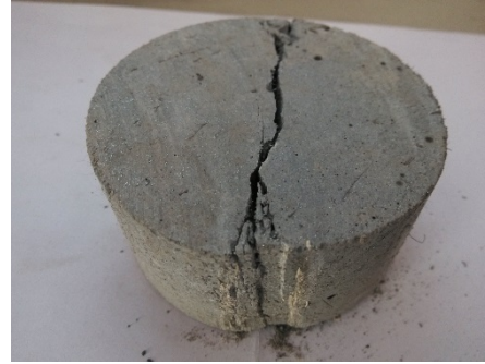
(b) Failure specimen
