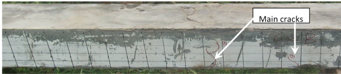
(b) UHPC Specimen with 1000 kN axial load under 17.5 kg charge weight loading
