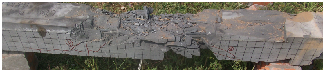
(a) HSC Specimen with 1000 kN axial load under 17.5 kg charge weight loading
