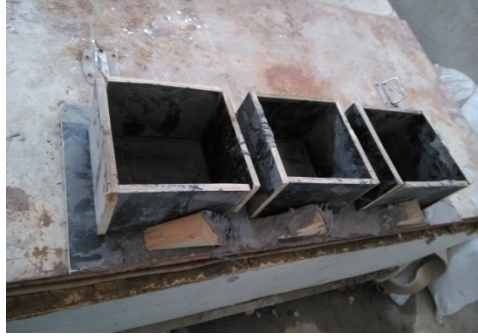
Figure 18: Concrete wooden moulds
