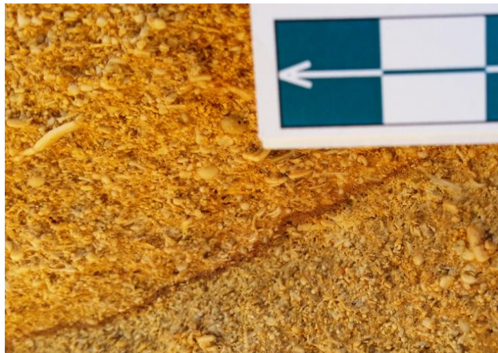
Figure 4) sharp micrite fill deformation band, hosting small amounts of individual bioclast grains.
