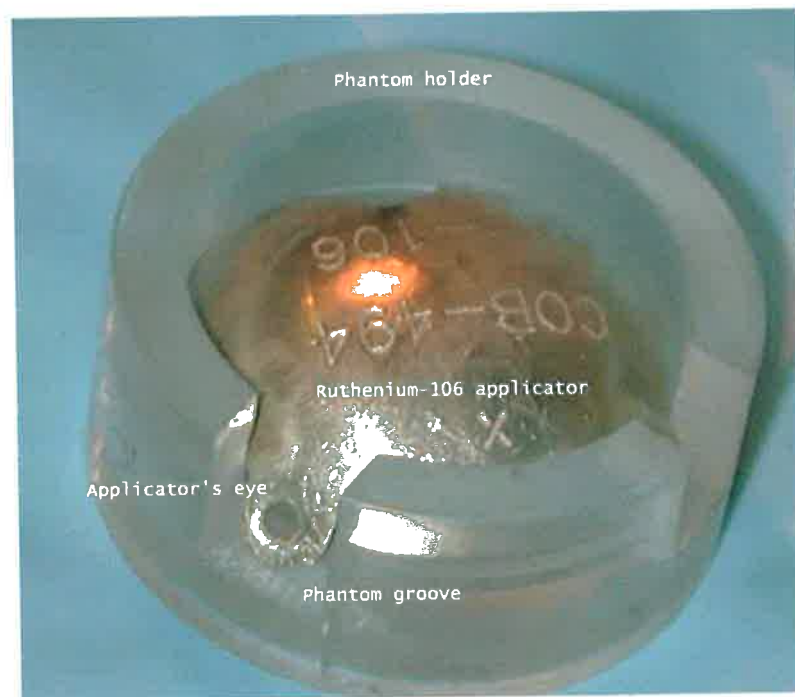
Figure 4.5 Position of the ruthenium-106 applicator on the eye phantom. As shown in the picture, both of the phantom slits firmly hold the applicator notches resulting in a firm positioning of the applicator.
