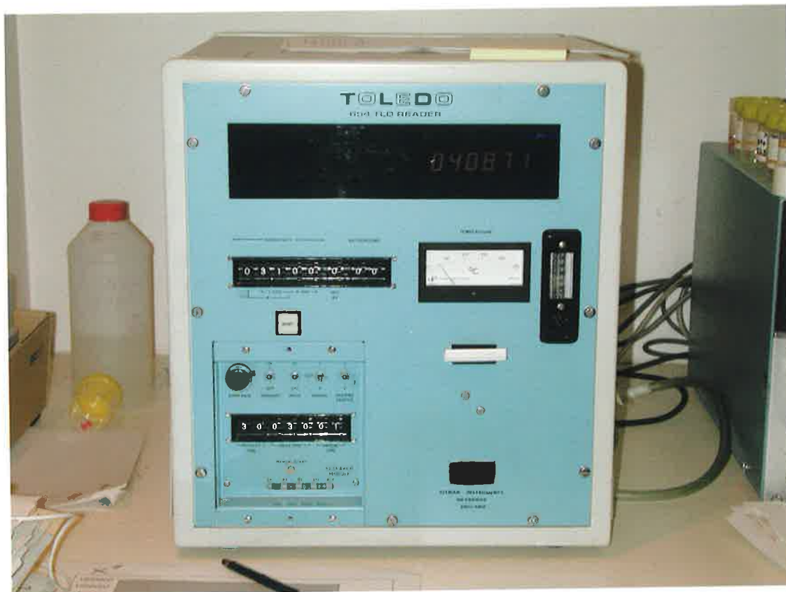
Figure 3.1 The front panel of the Toledo universal TLD reader (Vinten Instruments Limited, England) used in the research project.
