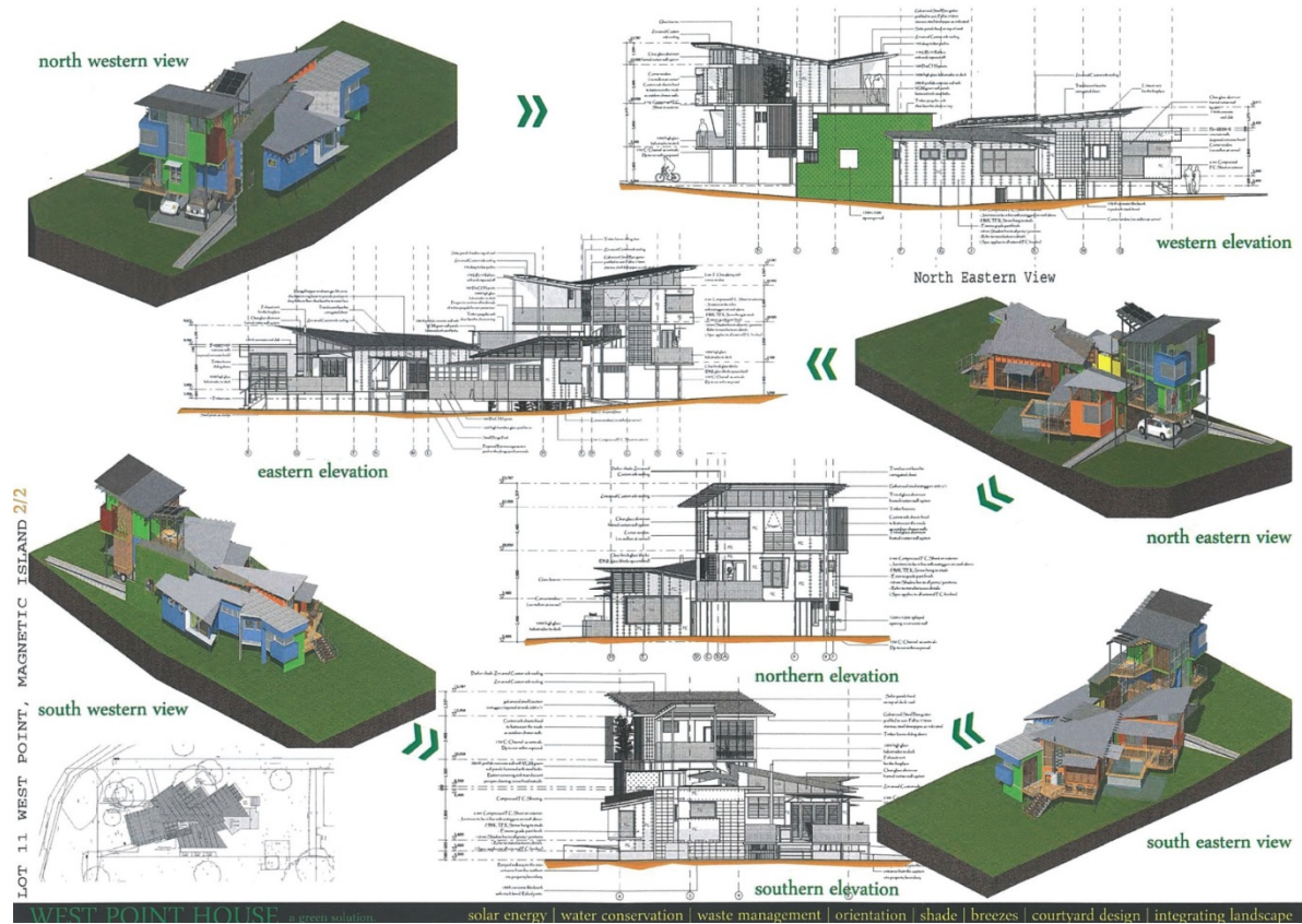
Figure 5.4f A house extension (Top) and a proposed house design (Bottom) represent O’Toole design concepts with complex elevations, irregular forms, various roof designs and composition of different volumes in various scales and layouts. O’Toole’s design approaches differ from Clark’s design concepts for simplicity.
