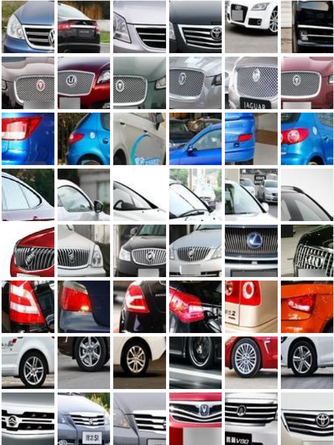
Figure 3.26: Patches with highest activations for several filters in the first convolutional layer (in total 64 filters) in the fine-tuned CompCars ResNet101-SWP. Each row refers to one learned convolutional filter. Six patches in one row represent the top six highest activations among all 14,939 test images. From the top row to the bottom are for the 5-th, 7-th, 17-th, 30-th, 34-th, 51-th, 54-th and 64-th filters.
