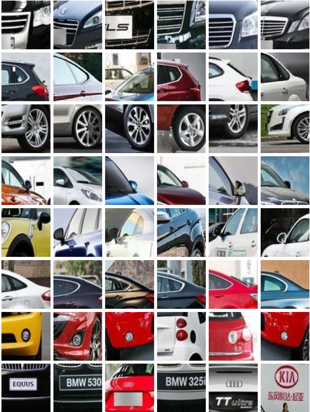
Figure 3.28: Patches with highest activations for several filters in the 6-th layer (in total 64 filters) in the fine-tuned CompCars ResNet101-SWP. Each row refers to one learned convolutional filter. Six patches in one row represent the top six highest activations among all 14, 939 test images. From the top row to the bottom are for the 1-th, 9-th, 13-th, 14-th, 15-th, 18-th, 49-th and 51-th filters.
