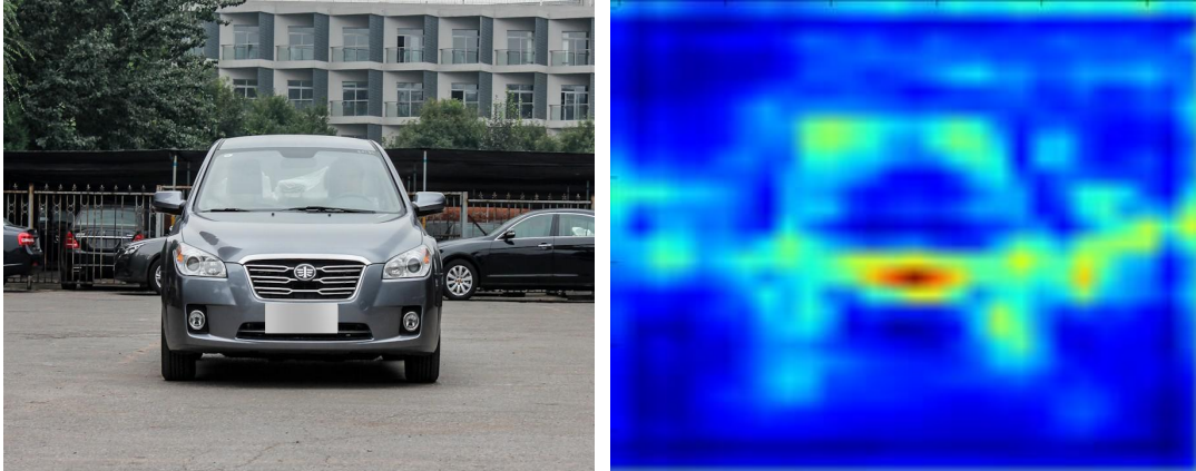
Figure 3.3: Visualizing of ROI regions by accumulating 512 feature maps of conv53 in the fine-tuned CompCars VGG model. Right: the original image. Left: the indicator map.
