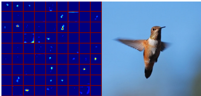
Figure 3.4: The first 81 of total 256 feature maps extracted from the last convolutional layer in AlexNet (left), and the corresponding input image (right).
