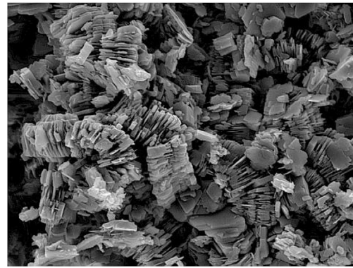
Fig. 2. Kaolinite particles attached to the grain surface (SEM image).
