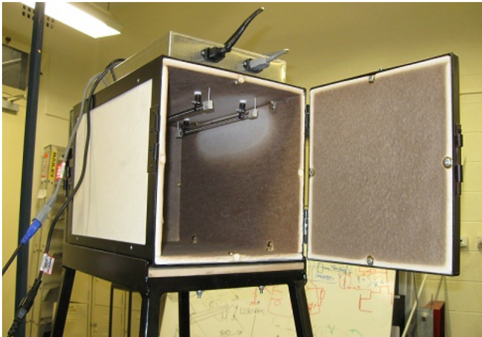
Figure 3-13: Halogen lamps in the dryer
