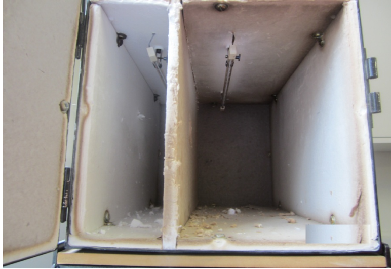
Figure 3-14: TITO furnace/dryer structure
