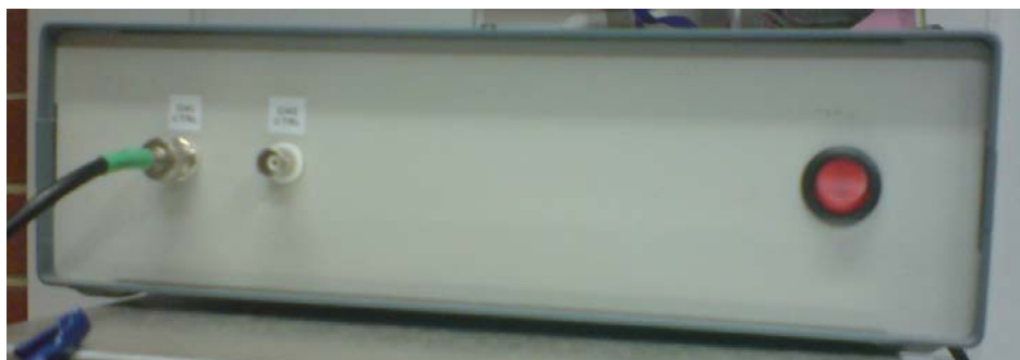
Figure 3-12: The power controller for the dryer lamps
