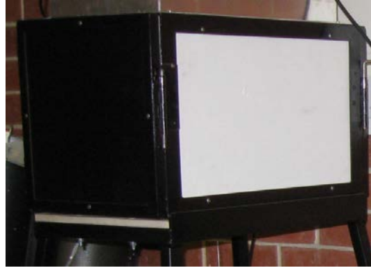
Figure 3-6: The walls of the dryer made by insulation boards and steel sheets
