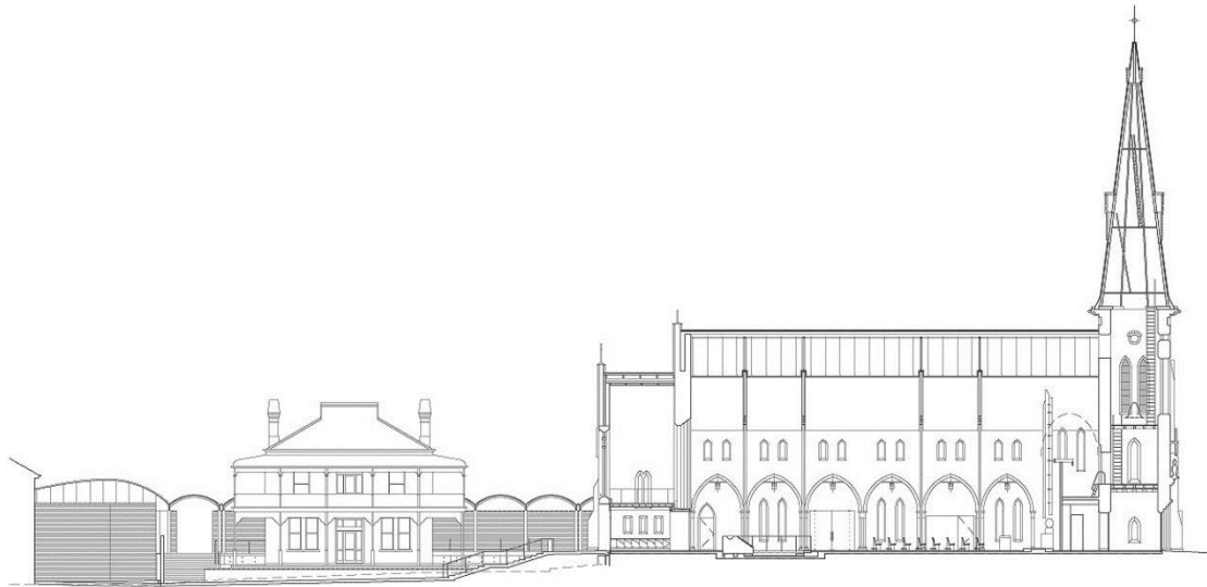
Figure 6.4 Section through Chapel showing the relationship to Murphy House. Guida Moseley Brown Architects.
