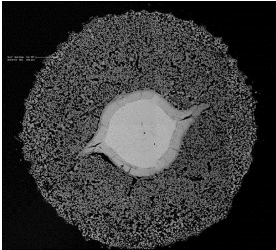
Figure 34 – BSC SEM image of a prepared cross section electrode captured on a Philips XL40 scanning electron microscope at an accelerating voltage of 15 kV
