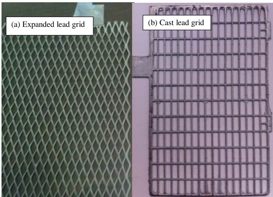
Figure 5 - (a) Expanded grid (Pacific Marine Batteries) (b) cast grid (Exide Technologies) illustrating modern lead grid designs compared to a thin flat sheet of lead used for grid in early development.
