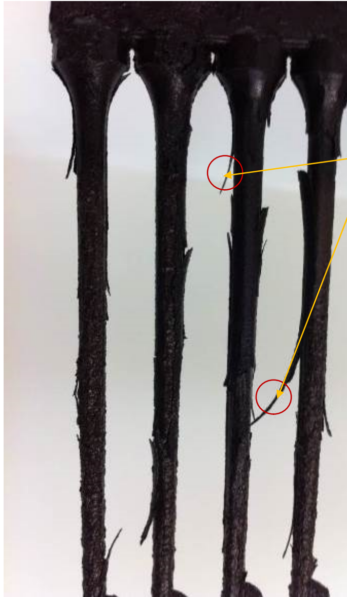
Figure 73 – shedding of the outer corrosion due to increase in corrosion product
