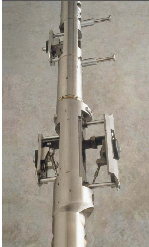
Figure 3-2 Modular dynamic tester (MDT) in multi-probe mode (Ireland et al., 1992).
