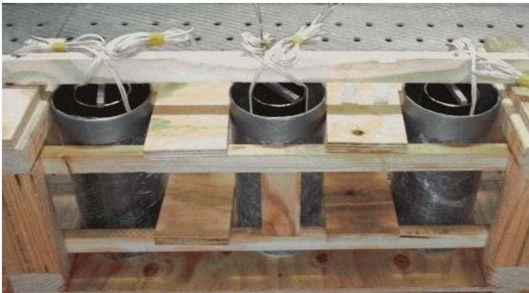
Figure 1. Formwork used in manufacture of DSTC specimens
