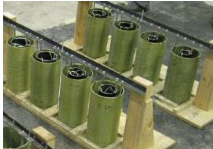
Figure 4. Formwork used in manufacture of DSTC specimens
