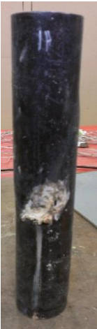
(a) Hollow D_s/t_s=60.3/3.6 (DSTC-1)
