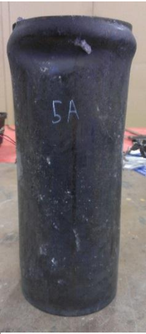
(e) Hollow D_s/t_s=114.3/6.0 (DSTC-9)
