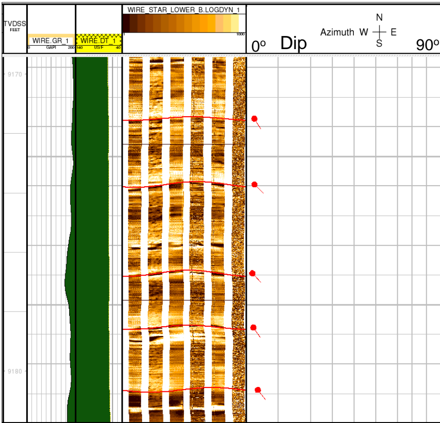
Figure 7.2: Example of sinusoids from dipping shale beds. The beds are dipping slightly (3-5°) towards 124°. This is equated to structural tilt of the interval, and is back rotated to horizontal for this section. Image pad 4 (far right) is noisy and is not able to be interpreted.
