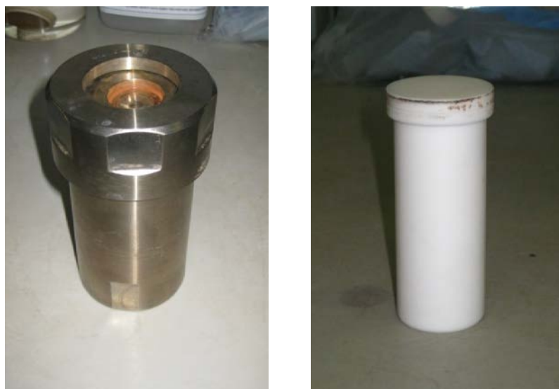
Figure 1. The stainless steel autoclave (left) that was used for silver sulfide nanoparticles synthesis and the Teflon® vessel insert (right).
