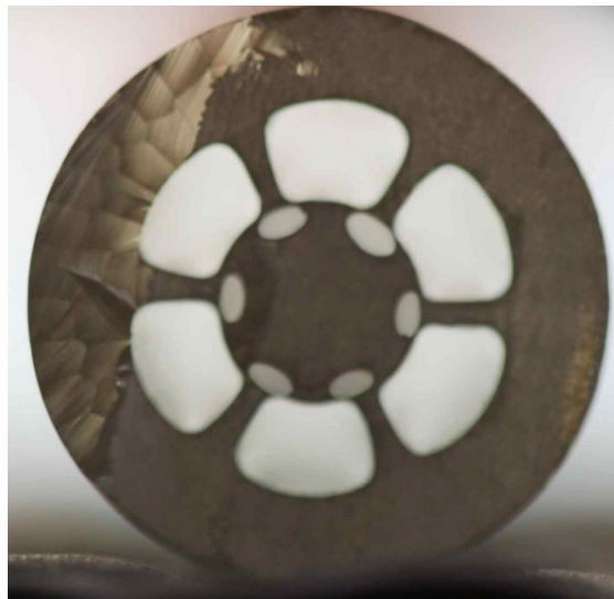
FIGURE 6.18: Results from Te-128 extrusion showing the preform fused into a solid block.
