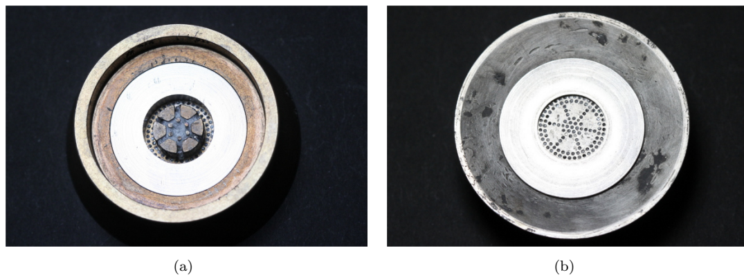
FIGURE 6.17: The v1.1 die. This die was made by taking the v1 die (pictured in Figure 6.12) and adding some modifications to block some of the outer feed holes and thus reduce the amount of glass flow in this region.
