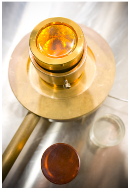
FIGURE 3.3: A cylindrical mould of the type in this picture is used to produce glass billets (seen at the bottom of the picture) for extrusion.
