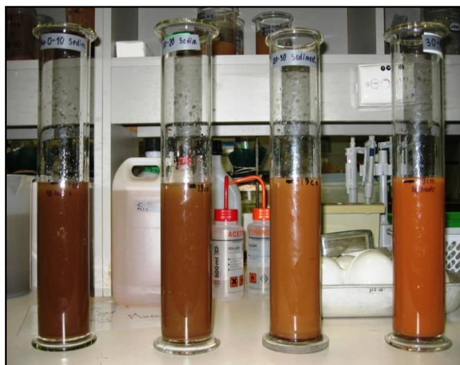
Figure 31 Settling of soil/water suspension of Urrbrae soil from cultivated (cereal) site for different depths, from the left: 0-10 cm, 10-20 cm, 20-30 cm and 30-40 cm
