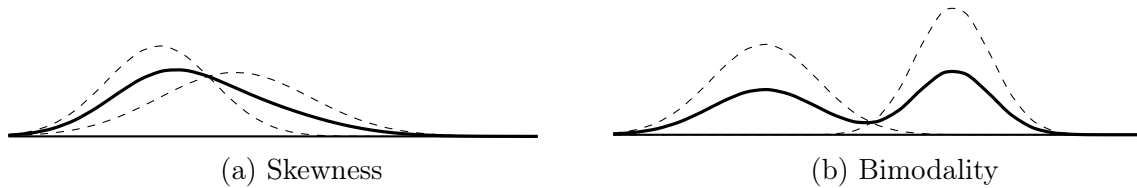
Figure 5.2: The probability density functions of two Gaussian mixture models in 1-dimension both using two equally weighted components. When individual components (dashed) are combined to produce non-Gaussian mixture densities (solid), they can exhibit both (a) skewness and (b) bimodality.
