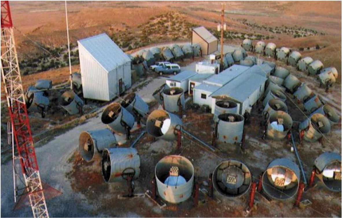
**Figure 2.9:** Fly's Eye I detector with mirrors mounted in steel drums with PMT arrays [35]
